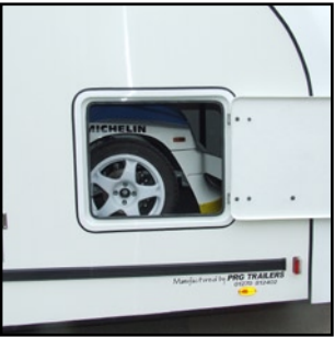
TIE HATCH/DOOR TO ENABLE TYING DOWN
